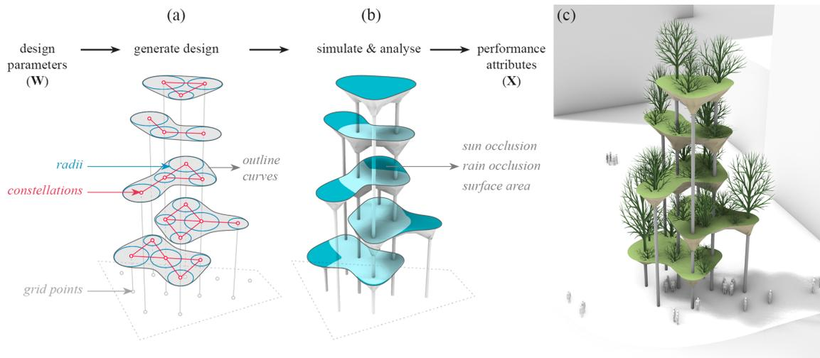
Figure 1: Process of parametric design, from the specification of the design parameters (a), the simulation of specific performance attributes (b), and the finally design achieved (c).
